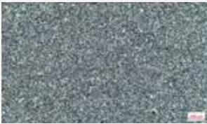
HOMOGEINITY OF EUTECTIC CARBIDE: LEVEL 0
